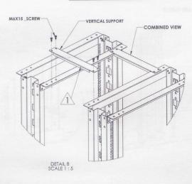
1) The vertical supports are fixed between the upper space of frames and to the holes on the horizontal supports by using M6x15 screws
