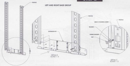
The front side of left frames which have square holes on it is fixed to the left base by using M8x15 screw , washer and nut . It is described as left profile and base group .
