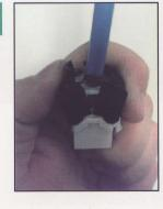
Close the outer cap by pushing down both sides of the outer cap until it clicks.
